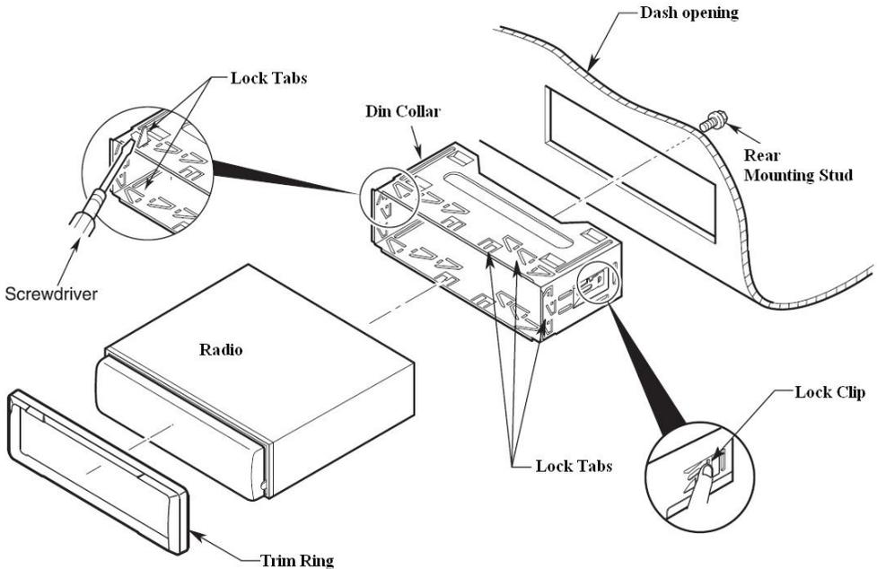
2. Route all cable through the DIN collar and make all the necessary rear connections with the radio. Verify clearance; then gently insert the radio into the DIN Collar until both sides are locked. Install Trim Ring if not already installed. Secure rear mounting stud for additional support if desired.
