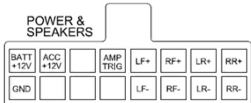
**\*WARNING:** Radio is designed for 12V DC negative ground systems only.
